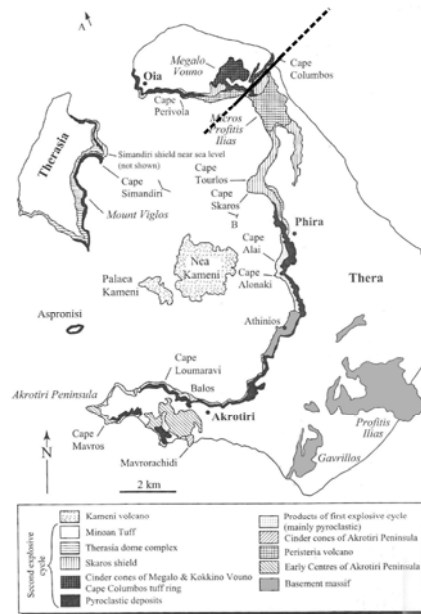
Figure 2. Geological map of the Santorini Islands; the heavy line represents the continuation of Amorgos fault (modified from Druitt et al., 1999).
