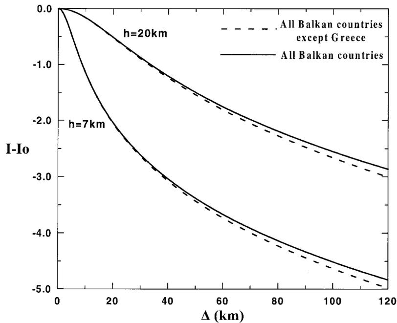
Figure 1. Comparison of the attenuation curve (solid line) determined for all Balkan countries by Papazachos and Papaioannou (1997) with the curve (dashed line) corresponding to all Balkan countries except Greece (present study). The attenuation curves are shown for two macroseismic depths (7 and 20 km).
