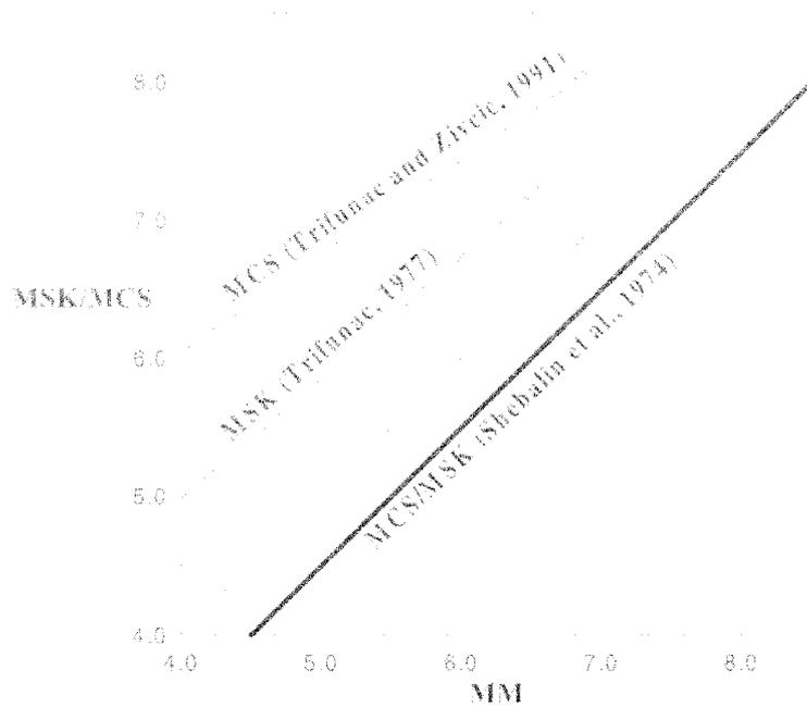
Figure 2. Comparison of the MCS–MM (Trifunac and Zivcic, 1991), MSK–MM (Trifunac, 1977) and MCS/MSK–MM (Shebalin et al., 1974) relations.
