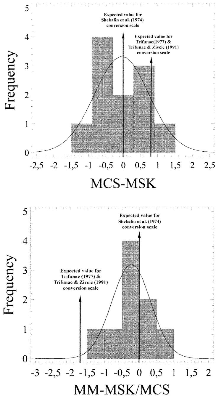
Figure 3. Distribution of the MCS-MSK and MM-MCS/MSK intensity differences computed in the present study after converting all intensity values to MM using Shebalin et al. (1974) relations. The best-fit normal distributions are also shown. The average difference is expected to be close to 0 if Shebalin et al. (1974) relations are valid. The expected difference for the relations of Trifunac and Zivcic (1991) and Trifunac (1977) are also shown.
