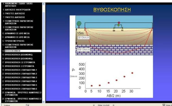
Fig. 3. Page of the web material of the course “Electric and electromagnetic prospecting methods” showing the current flow in the subsurface and the produced sounding curve [2].
